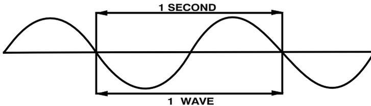
Often a reference is made to a stations wavelength rather than it's frequency. High frequency signals have short wavelengths and low frequency signals have long wavelengths. The frequency of a signal in kHz is given by dividing 300,000 by the wavelength in metres.
