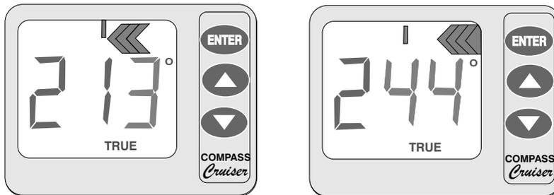
Figure 4a & 4b - Three and ten-chevron Steering indications
