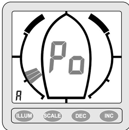
**Figure 5 - Engineering mode, Port tack vane position logged**
