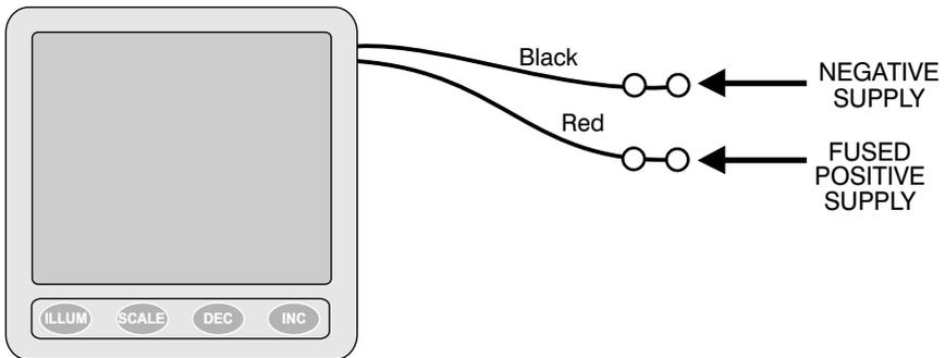
**Figure 1 - Wiring Installation**
